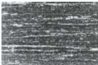
Conventionally produced HSS with a brittle carbide microstructure limits material strength.
