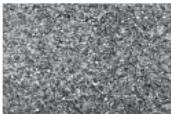
The fine, uniform microstructure of ASP® carbides ensures superior strength.
